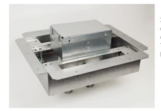
2-Gang Fire Classified Steel Floor Box. Adjustment range over deck of 2" (51mm) minimum to 5" (127mm) maximum. Two 1 1/4" (32mm) conduit feed openings. Box Capacity - 58.5 cubic inches per gang. This floor box preserves the 2-hour fire rating of floors in which it has been installed.
