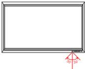
▶ Point the remote towards the remote control sensor of the wireless monitor and use it within 7 meters.
