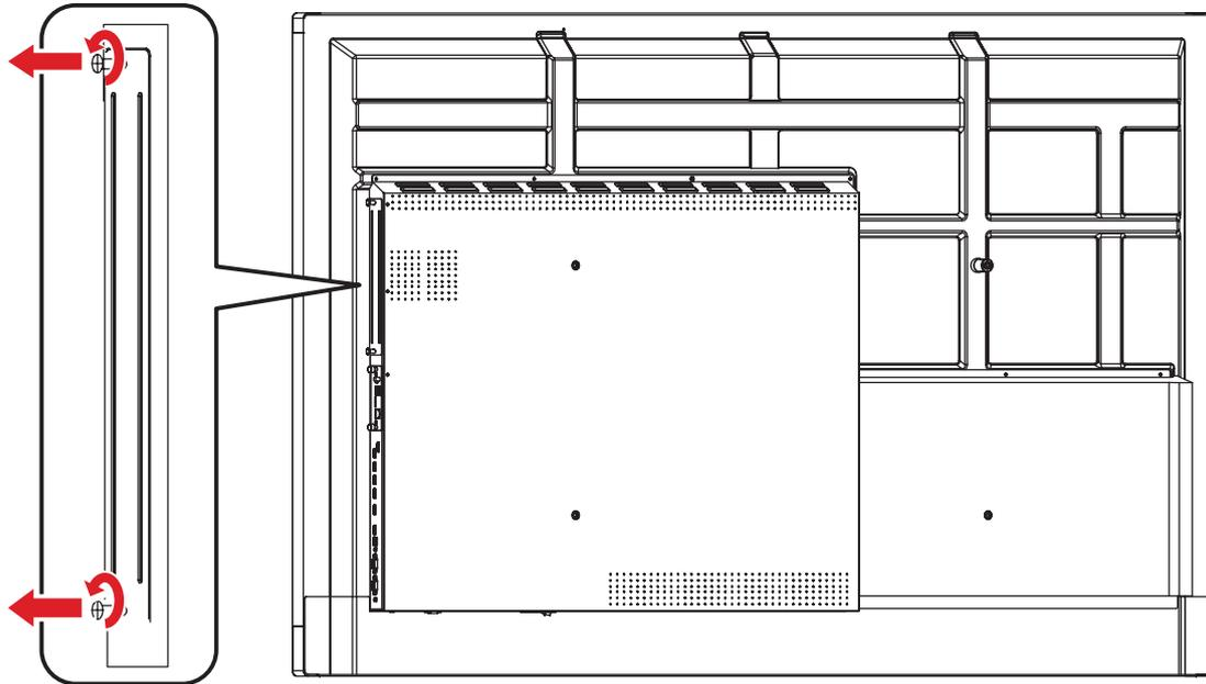
2. Carefully insert the VPC33/VPC35/VPC37 into the PC slot of the display.
