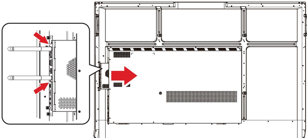
3. Secure the VPC33/VPC35/VPC37 to the display with the two (2) screws.
