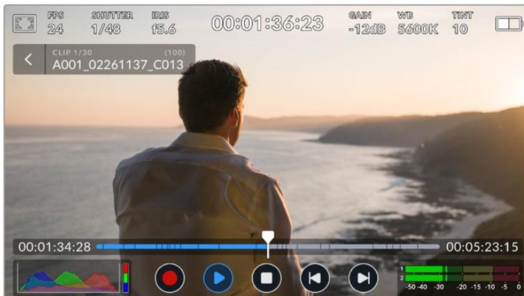
The LCD touchscreen displays a timeline of segments representing all the recorded clips. Each segment in the timeline represents an individual clip. The current clip name and number is shown at the top left of the display and the total number of clips on the card or drive is shown in brackets.
