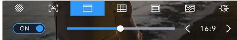
Tap the 'frame guides' icon while accessing 'LCD monitor options' to access your URSA Broadcast G2's frame guide settings
