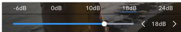
While in the 'gain' menu, your URSA Broadcast G2's gain settings appear along the bottom of the LCD touchscreen. The slider and arrows below the presets let you adjust the gain in 1/3 stop increments.
