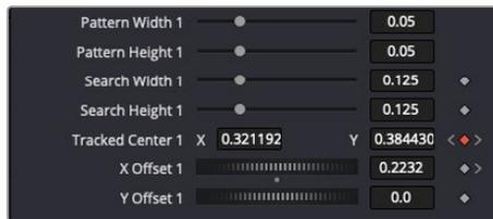
Scroll wheels at the bottom of the tracker inspector panel let you adjust the offset position for the text.
