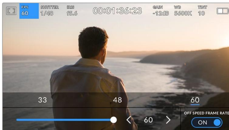
With 'off speed frame rate' enabled, tap a preset or the arrows on either side of the sensor frame rate or move the slider to make adjustments
