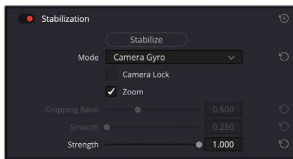
In the inspector window select 'camera gyro' to stabilize the footage using gyro data
