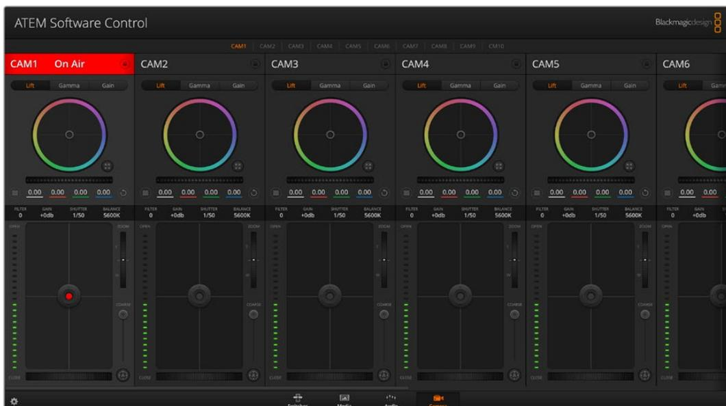
Try adjusting the iris and pedestal in ATEM Software Control's camera page to test camera control
