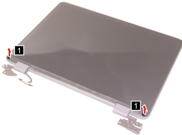
Figure 44. Remove the strip cover screw mylar
