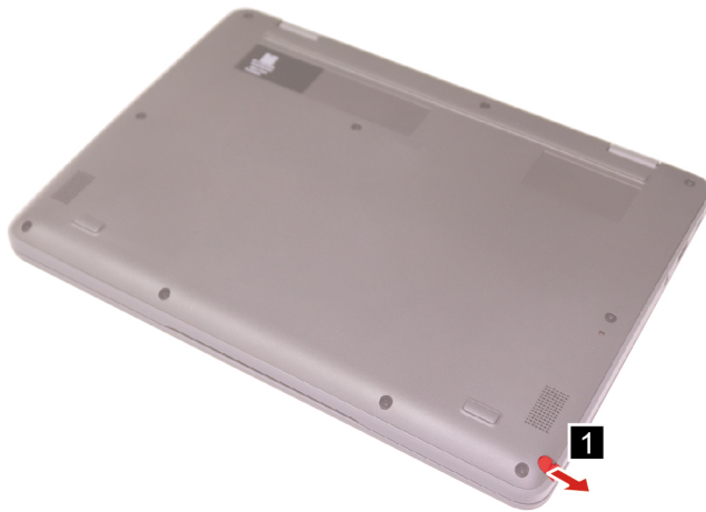
Figure 2. Remove the electronic pen
