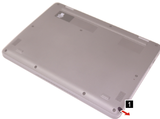
Figure 3. Remove the dummy pen cap
