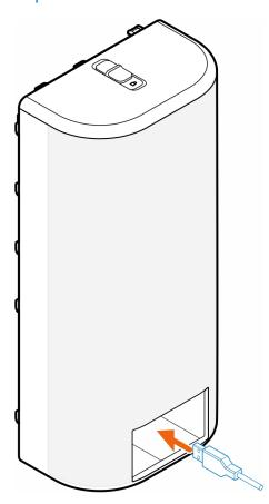
**3.** Connect the cables to their respective ports on the chassis.
