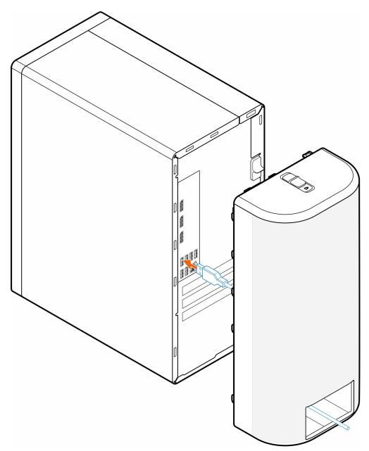
**4.** Align the cable cover retaining hooks with the slots on the chassis.
