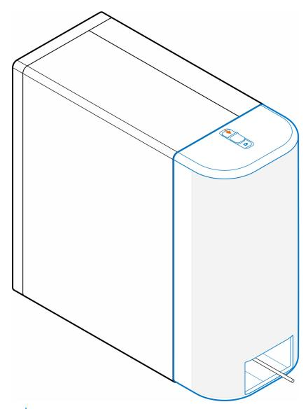
(i) NOTE: For added security, use the Kensington cable lock to secure the computer.
