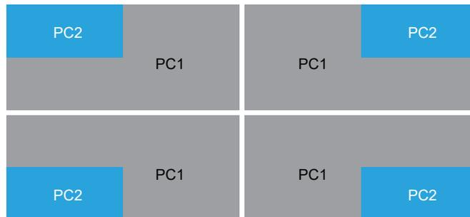
As same to PBP, the PIP (Picture-in-Picture) function can receive two different video sources too. The best resolution of foreground PC2 is 5120x1440@165Hz.
