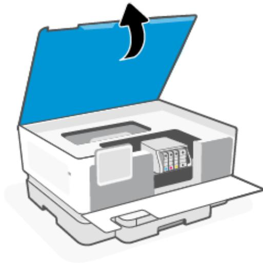
3. Look inside the printer and remove any jammed paper found. Move the carriage to the left and right to fully inspect the print area for any jammed paper.
