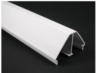
Used as a vertical corner feed drop to horizontal run of 5400 Series Raceways. Two compartments. Packaged with base and cover. MXN2A08 available in 8' (2.44m) lengths.
