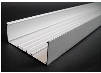
6063-T5 extruded aluminum, satin anodized finish, .080'' (2.03mm) wall thickness. Base has four ribs for snap-in divider. This base is packed eight 5' (1.5m) lengths per carton.
