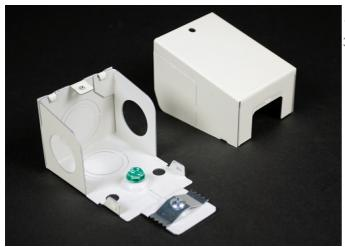
1/2" trade size KOs located on end, sides, and bottom of fitting. 3/4" KOs on bottom and rear. Includes ground screw.
