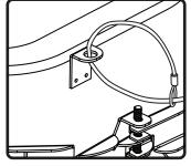
6. If required, a sheet-metal tab located on the rear panel of the speaker serves as a secondary point of attachment (cable not included).
