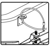
7. If required, a sheet-metal tab located on the rear panel of the speaker serves as a secondary point of attachment (cable not included).
