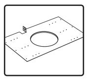
1. Nail or screw bracket to joists. Secure conduit/signal wire away from hole in bracket.
