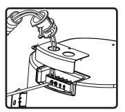
4. Run signal wires through conduit connector, then through cover plate. Connect to ceramic terminal strip. Two + and two - connectors are provided for daisy chaining.
