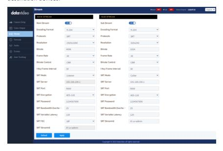
Caller and listener modes work together to establish the SRT link between source and destination devices. It is arbitrary to set one device to listener mode and the other to caller mode. Either can be the source device.
