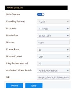
5. Click the **Apply** button to activate the RTMP video stream. Make sure both audio and video are enabled.
