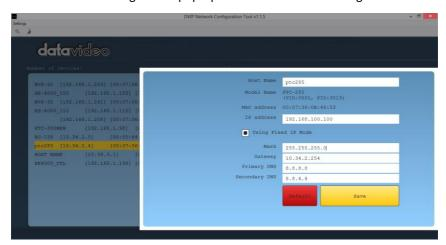
Step 4: You are allowed to change the device name in the Host Name field and modify the device's network settings accordingly. Click the Save button to confirm the change. To reset, simply click the Default button.
