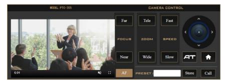
A preview window is positioned in the left half of the panel, allowing you to view the live camera video. Elapsed time is shown in the bottom left corner of the window. At the bottom right corner, click to enable sound. Use the sound slider that appears to adjust the volume accordingly. Click to view the video in full screen.
