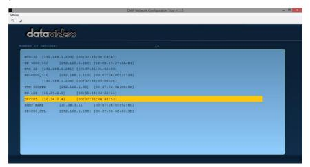
Step 3: Click one of the connected cameras to show the device information and its network settings in the pop-up window shown in the diagram below.
