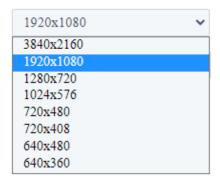
Adjusting the image size is a critical step of encoder setup. It is best to either match your original video source or scale it down. For example, capture at HD 720 and stream at HD 720. Or capture at 4K 2160 and stream at Full HD 1080.
