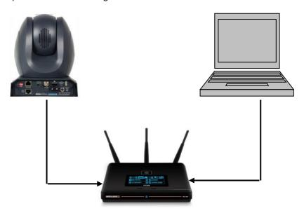
After connection has been successfully established, use DVIP Configuration Tool to search for the camera's IP address. If you are new to DVIP, see the **DVIP** section for more descriptions of the tool.
