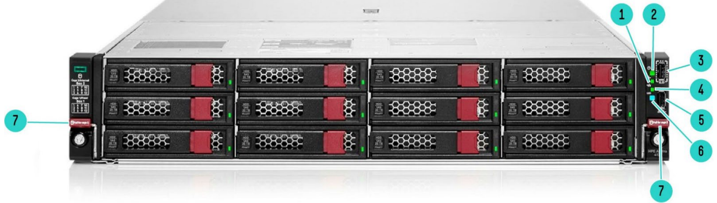
HPE Alletra Storage Server 4120 Configure-to-order System Front View (24LFF SKU shown)
