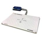
The XT-EF AirGesture sensors registers left, right, up, and -down swipes within the sensor's detection field. AirWheel detection processes circle tracing by the user's fingers above the sensor. The AirButton feature detects whenever a person's hand enters and leaves the sensor's detection field and can also register and respond to physical Touch input.
