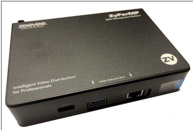
Installations will require a ZyPer Management Platform (ZMP). This device controls the operation and manages the connectivity between endpoints. The management platform is a hardened controller node that must reside on the same logical network as the ZyPer Encoders and Decoders. It runs a ZeeVee application as its sole function. The application presents an API to potential third party management platforms as well as hosting its own browser based management application.
