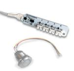
The X-Touch button interface is a 4-channel pushbutton interface with LED control and can be used in combination with industry-standard push buttons. It allows the connection of up to four buttons onto a single interface. This results in the connection possibility of up to 9 push buttons even on the smallest Xperience controller. Programmable LED output options are on, off, slow and fast blink.
