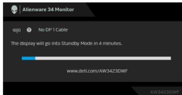
**📎 NOTE:** This dialog box also appears during normal operation, if the video cable is disconnected or damaged.
