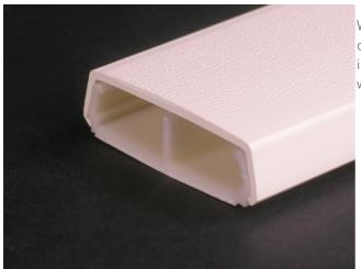
Wiremold 2300 Series Raceway is a low-profile, two-piece dual channel raceway with durable, textured PVC ivory finish. Available in 5' (1.52m) lengths. Packed 50' (1.5sm) per carton. Supplied with wide adhesive tape along its entire length.
