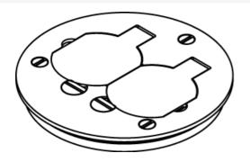
Brass duplex cover plate with flip lids, 4 1/4" (108mm) for tile. NOTE: For carpet or tile installations. All cover plates are furnished with gasket and three screws. The 895P Polycarbonate Series Cover Plates must be field modified for dual service.
