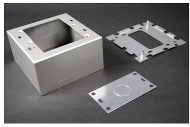
Two Gang Deep Device Box. For larger receptacles and deep devices such as those of signal and alarm systems. Base has open black plate for mounting to existing wall box and solid black plate insert with 1/2'' and 3/4'' trade size Kos to close opening. Accepts industry standard faceplates for communication devices. Aluminum
