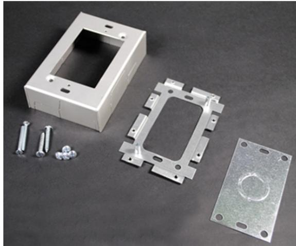
Designed for standard shallow switches and receptacles. Base has open back plate for mounting to existing wall box and solid black plate insert with 1/2" and 3/4" trade size Kos to close opening.
