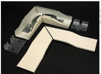
90 degree flat corner elbow provides 2'' (51mm) cable bend radius for fiber optic and UTP/STP cable installations. Ideal for lay-in or pull-through installations. Couplings included.
