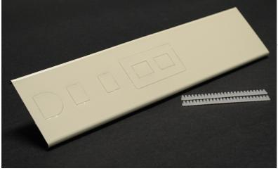
For 30TP-2V / 30TC-2V and 30TP-4V / 30TC-4V Series. 12" (305mm) long. Communication covers for additional voice/data connectors. Each cover includes Kos for four RJ11/RJ45 connectors (.760" x .576" (19.3mm x 14.6mm)), mouse hole for exiting communication cables (grommet furnished).
