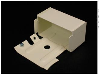
Connects 3000 Series Raceway with 1/2" trade size conduit and armored cable connectors. 1/2" trade size KOs on end and each side of fitting. Can be connected to conduit boxes by using 1/2" chase nipple.
