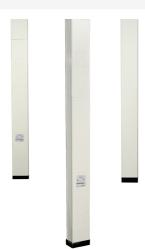
Single-compartment pole. Nominal material thickness .040" [1.0mm]. Furnished unwired without outlets. Mounting hardware, entrance end fitting and ceiling trim plates furnished. Length: 10'5" [3.2m].
