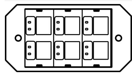
Single-gang device plate that will accept up to six (6) ports of communication devices. Fits in any one (1) of the three (3) gangs in the center compartment. Devices supplied by others.
