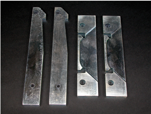
Case hard steel replacement blades and die set for 630C Cutter.
