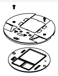
Nonmetallic slide holder assembly. Available in gray (GY), black (BK), ivory (VY), aluminum colored (AL) and brass colored (BS). NOTE: Assembled with scrub water gasket. For use on tile or carpet floors. AV3 Series Poke-Thru Devices require a 4" (102mm) diameter hole. Not designed to work with bare concrete or terrazzo. Floor covering thickness 1/8" minimum.
