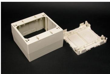
Two-gang. Base has rectangular KO to enable extension from existing single-gang flush wall box and 1/2" and 1" trade size concentric KOs. Accepts industry standard faceplates for switch and communication devices.
