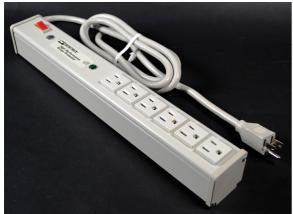
Sentrex high performance surge protection. Six outlets, lighted switch, durable putty white aluminum housing, 15A. 6' (1.8m) 14/3 SJT putty white cord with NEMA5-15 plug. Length 15 1/4"" (387mm). Snap-on, slide-off mounting.
