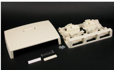
Fiber storage loop. Accepts three CM2 size Wiremold Open System communication modules or Pass and Seymour Activate Series inserts. Compatible with Wiremold 400, 800, and 2300 Series Raceways.
