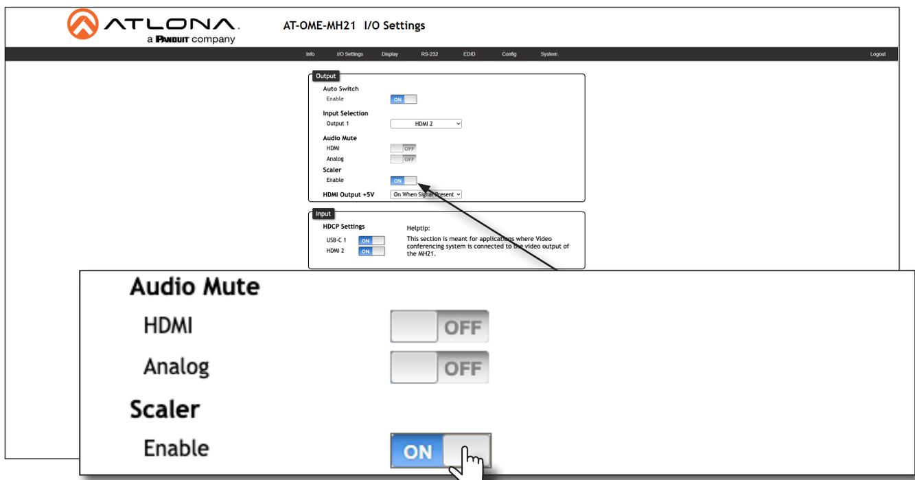
The screenshot shows the AT-OME-MH21 I/O Settings page. The 'Scaler' toggle switch is currently set to 'ON'. A red box highlights the 'Scaler' section, and a magnified view below shows the 'Audio Mute' and 'Scaler' sections. The 'Audio Mute' section has 'HDMI' and 'Analog' toggles set to 'OFF'. The 'Scaler' section has the 'Enable' toggle set to 'ON'.
