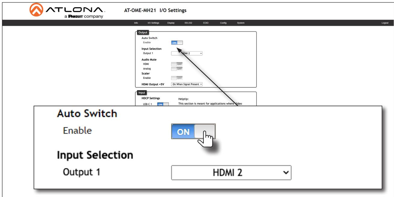
The screenshot shows the AT-OME-MH21 I/O Settings web interface. The 'Output' section includes the following settings:
