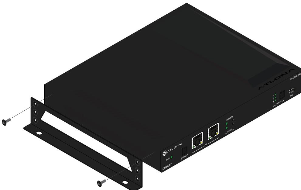
4. Repeat steps 1 and 2 to attach the second mounting bracket to the opposite side of the unit.
