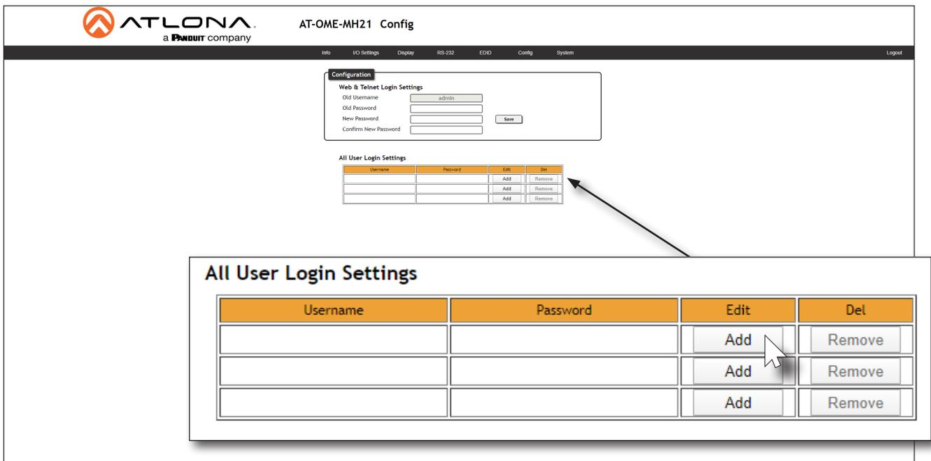
The screenshot shows the AT-OME-MH21 Config web interface. At the top, there is a navigation bar with 'Info', 'IO Settings', 'Display', 'RS-232', 'EDID', 'Config', and 'System'. Below this, there is a 'Configuration' section with 'Web & Telnet Login Settings' containing fields for 'Old Username' (admin), 'Old Password', 'New Password', and 'Confirm New Password', along with a 'Save' button. Below that is the 'All User Login Settings' table:
