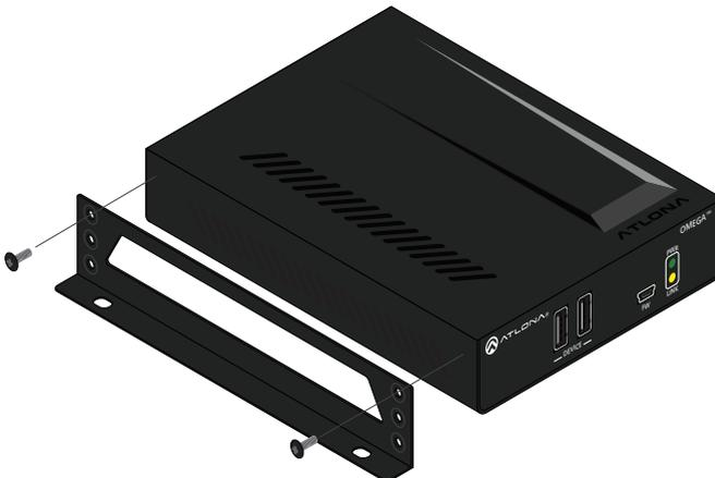
4. Repeat these steps to attach the second mounting bracket to the opposite side of the AT-OME-EX-RX-LT.
