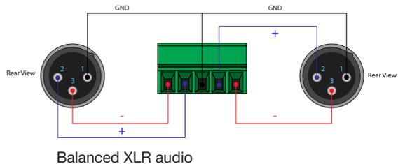
**i** **NOTE:** If unbalanced audio is needed, then it is recommended to use a stereo balanced to unbalanced converter.
