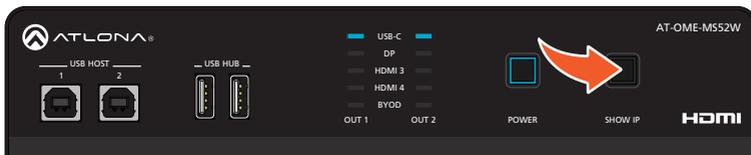
4. The IP address and the subnet mask of the AT-OME-MS52W will be displayed in the lower-left corner of the display, as shown below.
