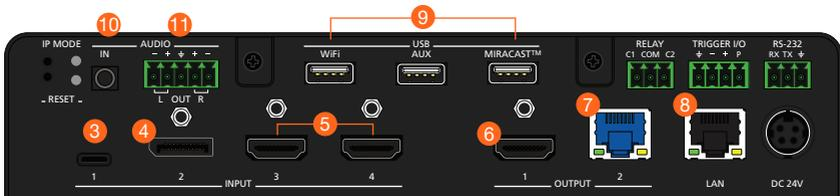
12. OPTIONAL: Connect the relay leads from the control motors of the projection screen, blinds, or curtains, to the relay outputs to the **RELAY** port, using the included 3-pin captive screw connector. Use a 48 V DC relay with no more than 1 A current draw. Refer to [Relay \(page 5\)](#) for wiring information.
