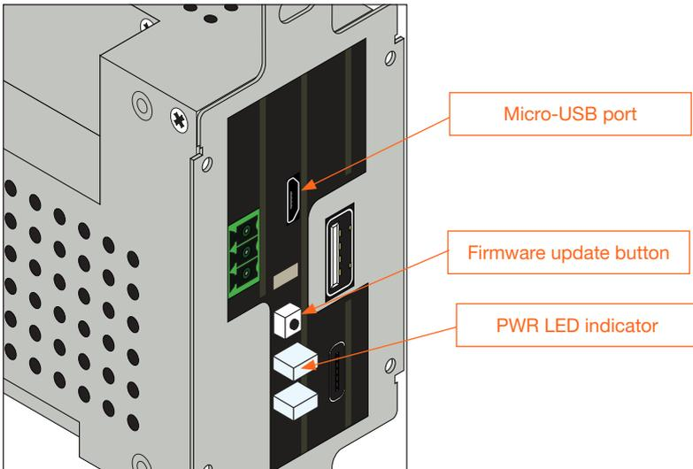
3. Connect a micro-USB to USB-A cable between the PC and the micro-USB port on the unit.
