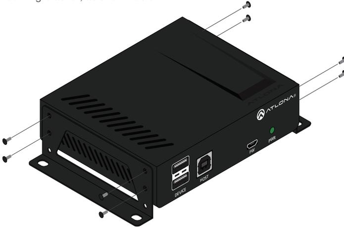
4. Mount the unit to a flat surface using the oval-shaped holes, on each mounting bracket. If using a drywall surface, a #6 drywall screw is recommended.
