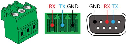
Pin out will be determined by the RS-232 cable and connect as RX (receive), TX (transmit) and  $\perp$  (Ground).
