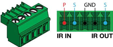
**IR IN** is connected by a power, ground, and signal wire. Use a 12V IR receiver with it (e.g. AT-IR-CS-RX purchasable through [atlonac.com](http://atlonac.com)).
