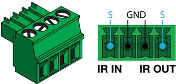
**IR IN** is connected by a ground and signal wire. Use with 3rd party control systems. For easy termination, Atlona recommends using the 2 meter IR cable AT-LC-CS-IR-2M (purchasable through [atlonac.com](http://atlonac.com)).
