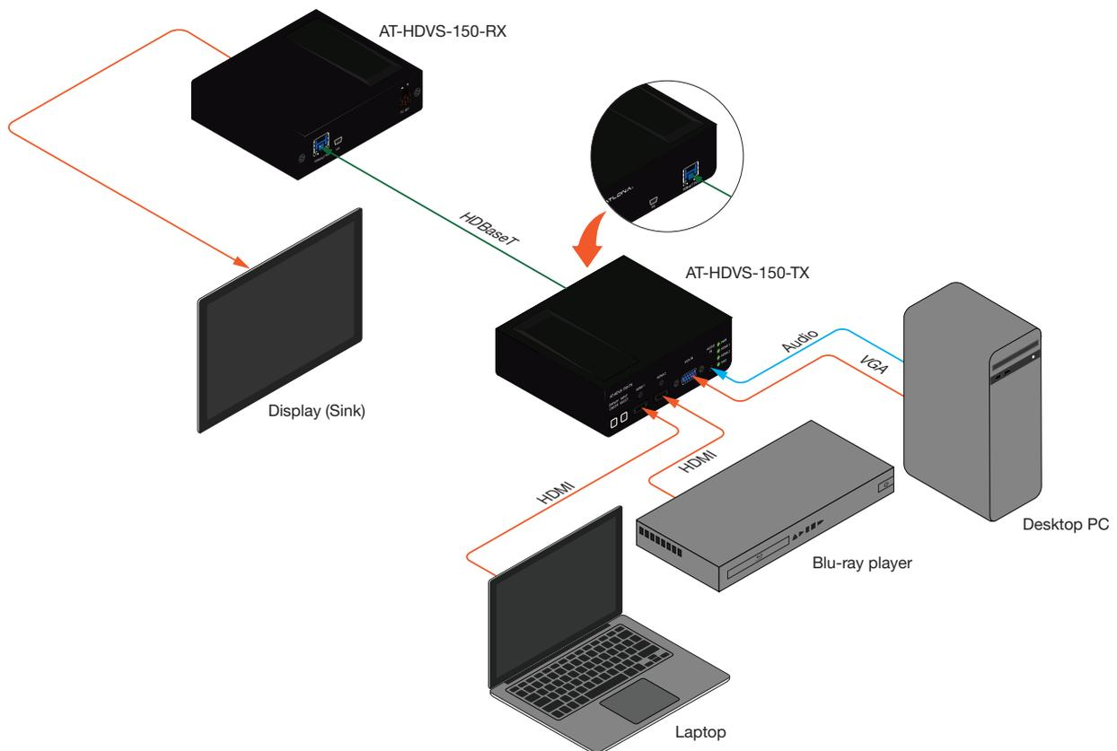
**i** **NOTE:** The AT-HDVS-150-RX is designed to be used with the AT-HDVS-150-TX.
