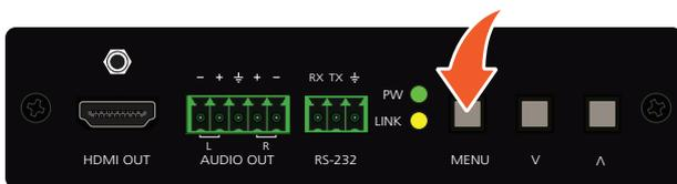
4. While pressing the **MENU** button, connect the USB cable from the computer to the **FW** port on the AT-HDVS-150-RX. When the USB cable is connected, the **PWR** LED indicator will glow solid green.
