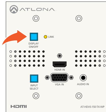
**NOTE:** When the display is in the “off” state, the **DISPLAY ON/OFF** button will glow bright blue. This functionality is added to assist in locating the wall plate in a darkened room.
