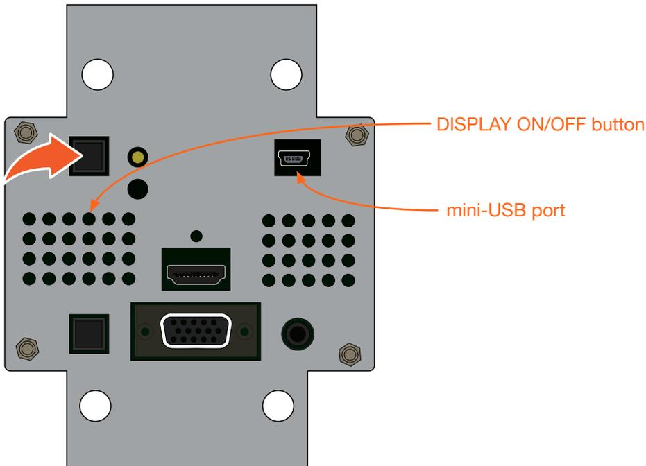
6. After a few seconds, a folder with the name USB UPDATER, will be displayed. Release the **DISPLAY ON/OFF** button.
