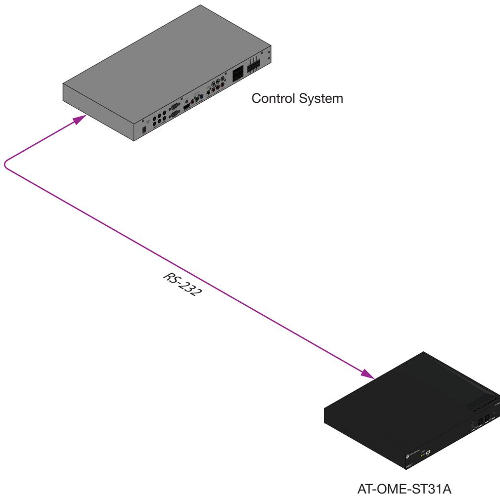
1. Connect a serial cable from the **RS-232** port on the AT-OME-ST31A to the RS-232 port on the control system. The included 3-pin captive screw connector should be wired as shown.
