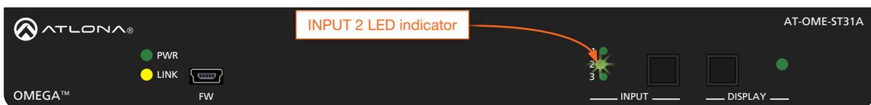
2. Press the **INPUT** button again to switch to **INPUT 3**.
