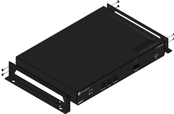
5. Mount the unit using the oval-shaped holes, on each mounting bracket. If using a drywall surface, a #6 drywall screw is recommended.
