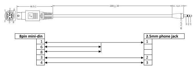
Warning: The 8pin snap-and-lock mini-din connector of the remote cable will be securely fastened once plugged into the Remote port. To remove, use two fingers to gently hold the part of the plug labelled by two arrows then pull the connector outward.
