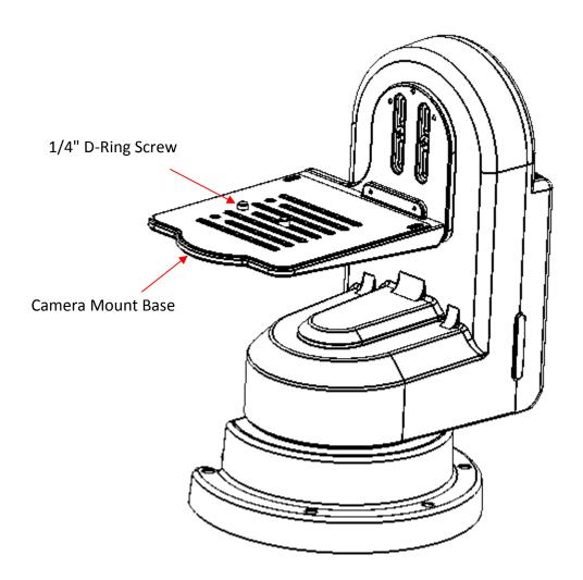
Note: It is recommended to use a flat head screwdriver to tighten the 1/4" D-ring screw as this can more effectively secure the screw.
