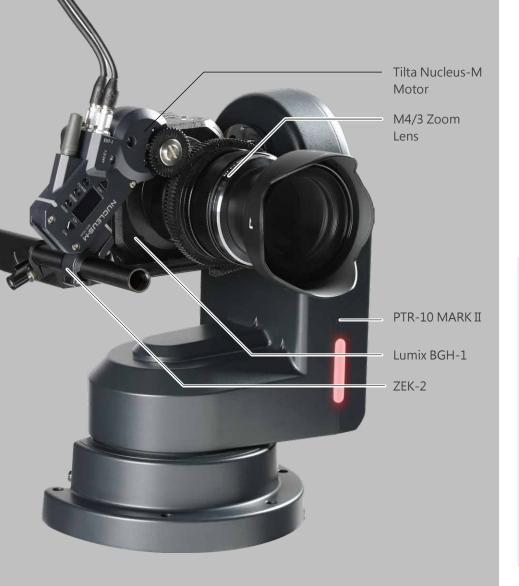
Through standard LanC protocol, PTR-10 MARK II can control the Focus and IRIS of the M4/3 Lens mounted on Lumix BGH-1. With the help of the Tilta Nucleus-M Motor Kit, we can also control the Zoom function of this camera. Even to recall the pre-stored zoom position.
