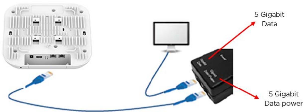
Figure 2: Installation of Enterprise Wi-Fi AP to a PoE adapter
