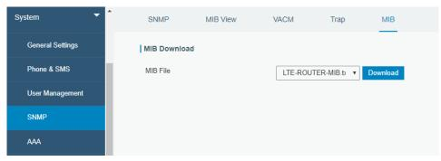
2. Start "ManageEngine MibBrowser Free Tool" on the PC. Click "File > Load MIB" on the menu bar. Then select "LTE-ROUTER-MIB.txt" file from PC and upload it to the software.
