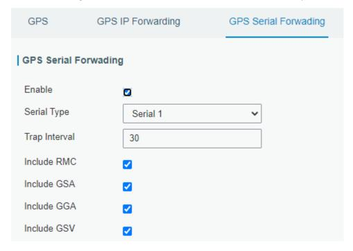
**Enable** Forward the GPS data to the pre-set serial port.
