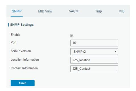
**Enable** Enable or disable SNMP function.
