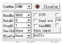
8. After connection is established between the iSite and the TCP server, you can send data between sscom and Netassit.
