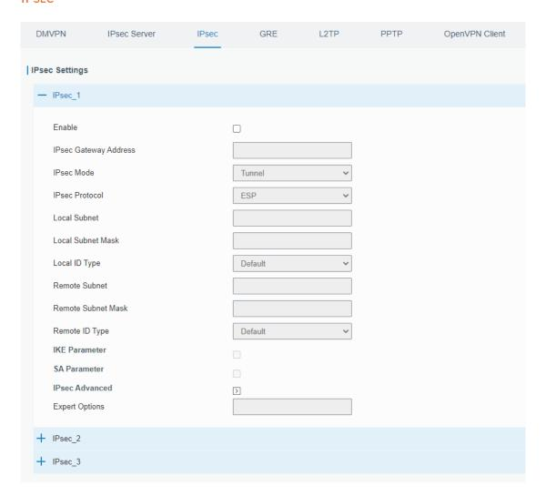
**Enable** Enable IPsec tunnel. A maximum of 3 tunnels is allowed.
