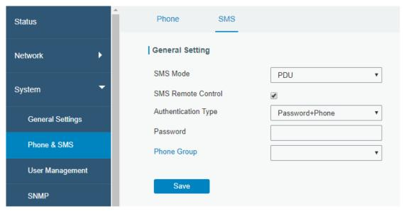
SMS Mode Select SMS mode from "TEXT" and "PDU".
