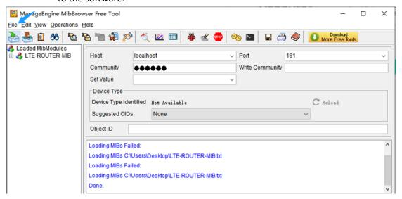
3. Click the "+" button beside "LTE-ROUTER-MIB," which is under the "Loaded MibModules" menu and find "usCellularinfo." And then you will see the OID of cellular info is ".1.3.6.1.4.1.50234", which will be filled in the MIB View settings.
