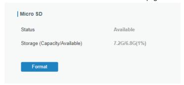
Status Show the status of Micro SD card, such as "Available" or "Not Inserted." Storage (Capacity/Available) The total capacity of the Micro SD Card. Format Format the Micro SD card.
