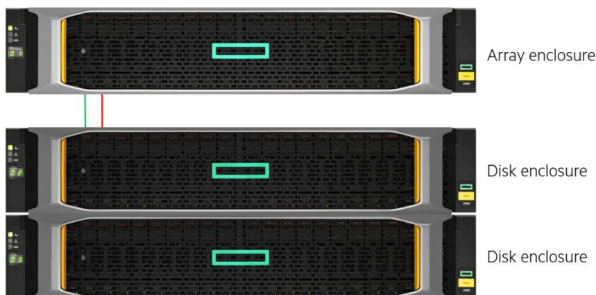
Figure 4. HPE MSA array and expansion enclosures
