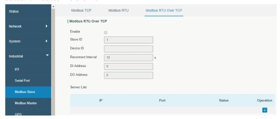
**Enable** Enable/disable Modbus RTU over TCP function.
