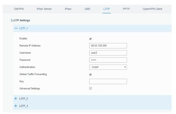
**Enable** Check to enable L2TP function.
