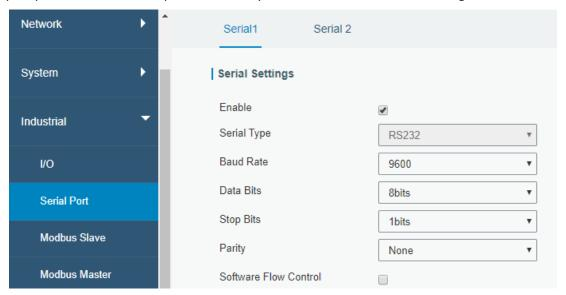
2. Configure Serial Mode as "DTU Mode." The iSITE is connected as client in "Transparent" protocol.
