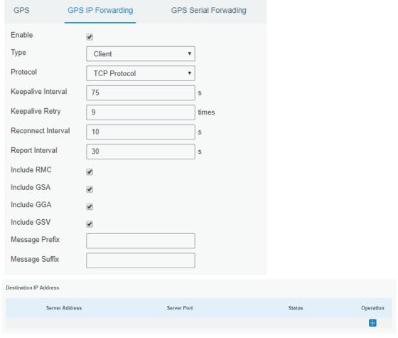
**Enable** Forward the GPS data to the client or server.
