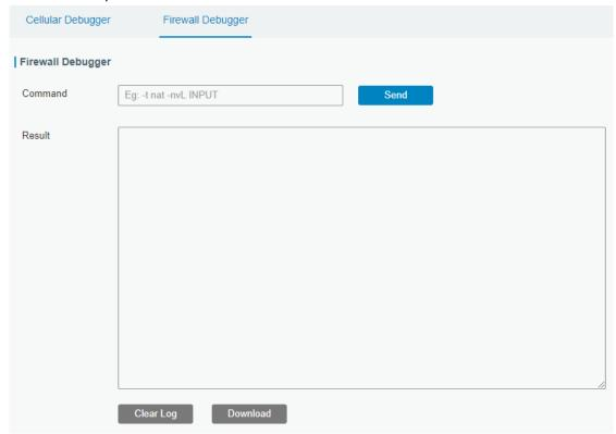
**Command** Enter the AT command that you want to send to firewall module. **Result** Show the response result from firewall module.
