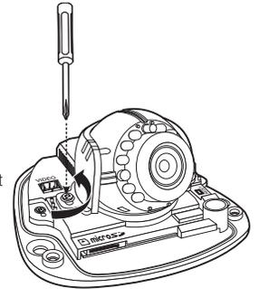
4. Adjust the lens in a desired direction by referring to the "Adjusting the monitoring direction for the camera" section. (page 10)
