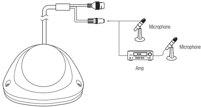
1. Connect the AUDIO IN port of the camera with the microphone or LINE OUT port of the amplifier that the microphone is connected to.
