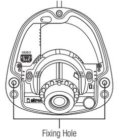
3. Turn the screws on both sides of the camera lens cover counterclockwise to loosen them.
