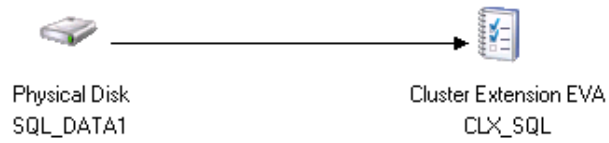
Figure 5. Physical disk resource SQL_DATA1 depends on the HP CLX EVA resource CLX_SQL
